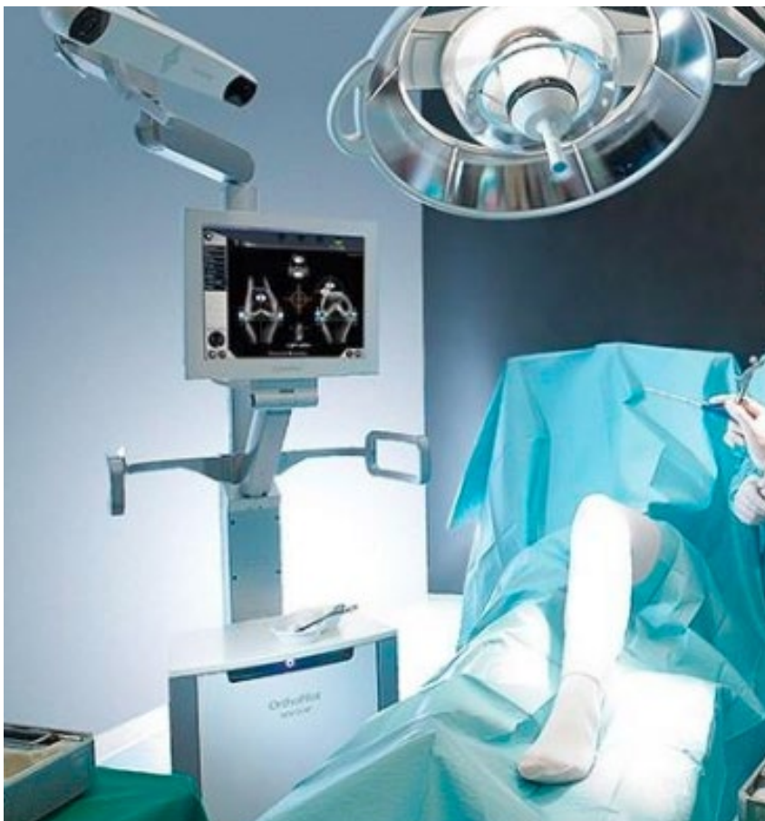
Slika 5. Orthopilot navigation system. Izvor: https://www.omnia-health.com/product/orthopilot%C2%AE
